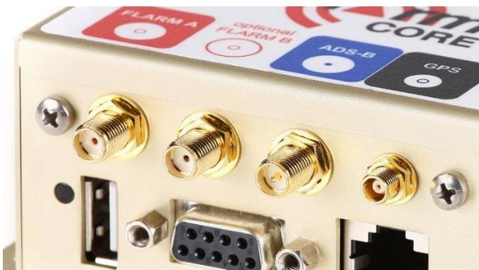
E-version devices (part No. FLAPFCnnE and FLAPFDnnE): FLARM A and B ports are standard female SMA connectors with a female center sleeve. ADS-B is a reverse polarity female SMA connector with a pin as a center conductor.
