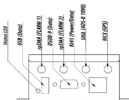
PowerFLARM Core has the following connectors:
